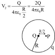
Therefore, net potential at P,  $V = V_1 + V_2 = \frac{q}{4\pi\epsilon_0 R} + \frac{2Q}{4\pi\epsilon_0 R}$
